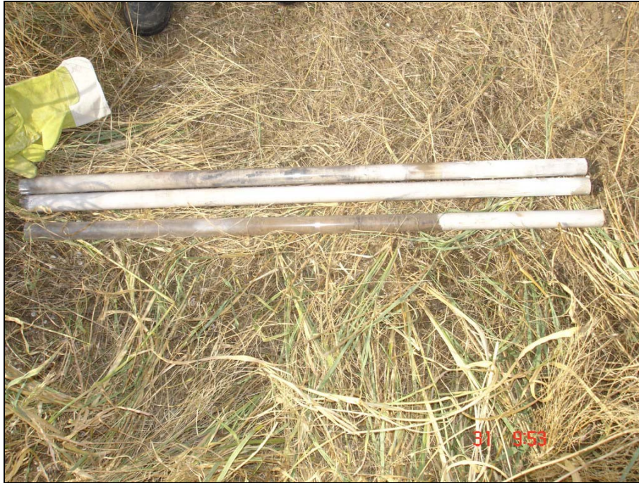
Figure 3: Drilling core at the dumpsite of \alpha - and \beta - isomers of HCH (white substance – waste isomers of HCH)
